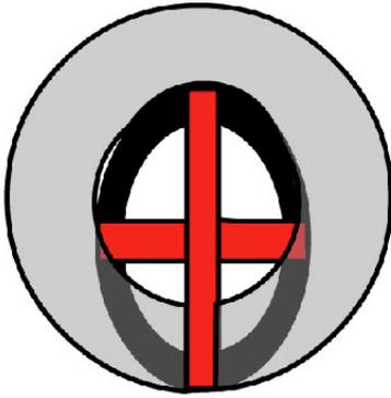
10. Put a rod like shown in the picture thru the runflat and remove the last compressor you set. (Take dish soap to make the rod sliding through).
