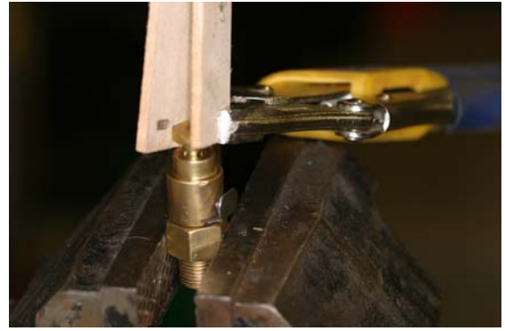
Figure 5 (Left) Cylindrical body housing removed (Right) Removal of brass seating disk
