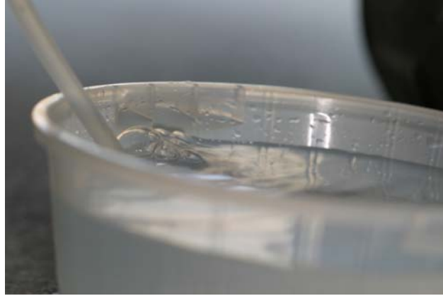
Figure 1 (Left) shows the test hose attached to the vent on the geared hub. (Right) the end of the hose is placed under water. You can see active bubbling due to a spindle seal leak.
