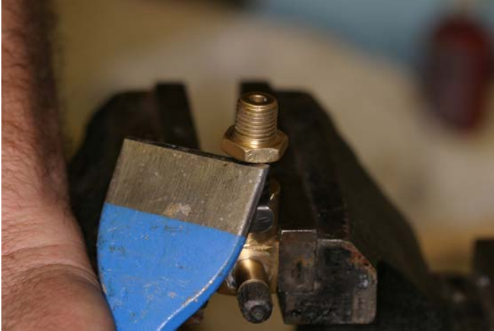
Figure 3 (Left) Placement of the chisel for old style valves.
