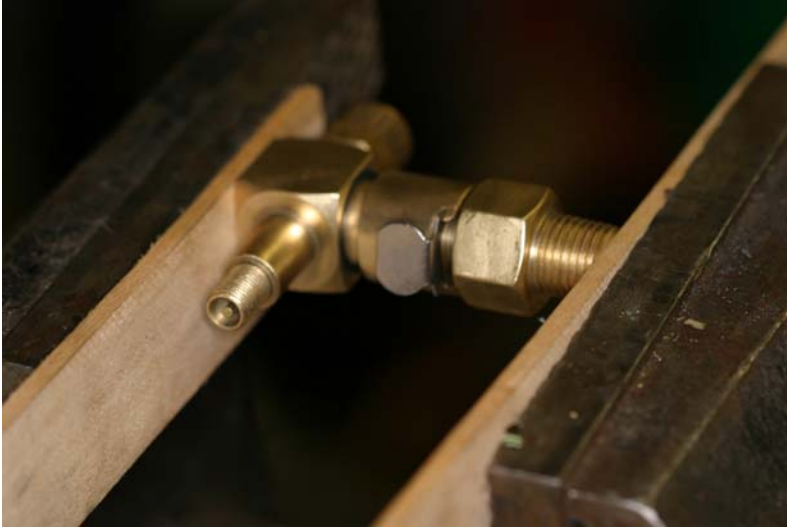
Figure 7 Using a vise to press in the valve body components.
