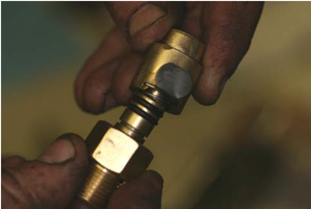
Figure 6 (Left) Press in the tab, separate the two components and remove the spring. This exposes the O-rings on the main shaft that tend to cause valve leaks.
