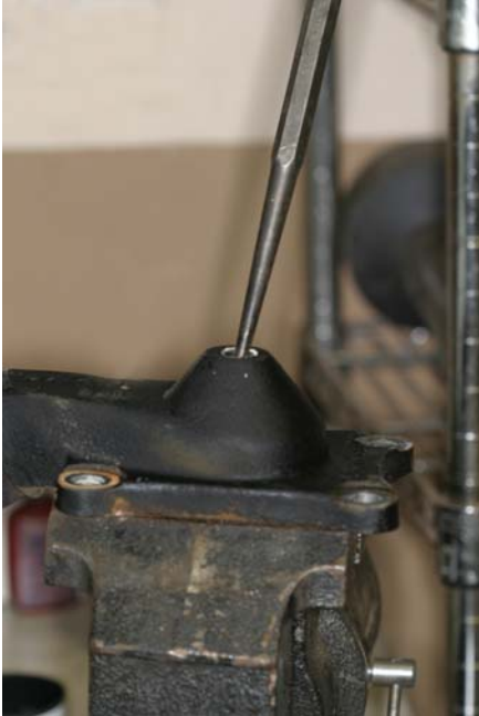
Figure 10 (Above) Using a long punch, catch the edge of the seal and hit the punch briskly with a hammer to unseat it.
