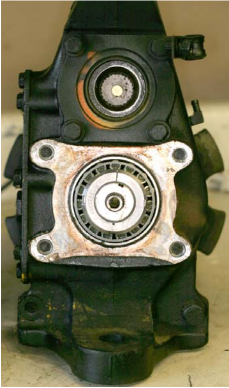
Figure 8 (Left) The Hub with the control arm plate removed. This exposes the clamp nut that holds the spindle. Above this is the exposed halfshaft input seal.
