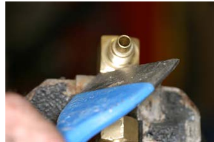
Figure 4 (Left) Location for placement of the chisel on new style valves. (Right) Chisel in position.
