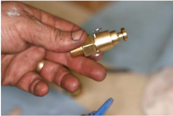
Figure 5 (Left) Cylindrical body housing removed (Right) Removal of brass seating disk
