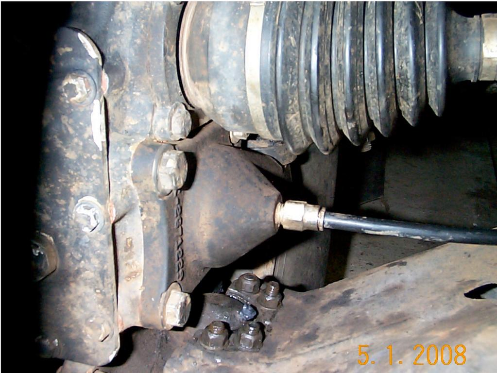
Quick connect fitting and nylon air line
