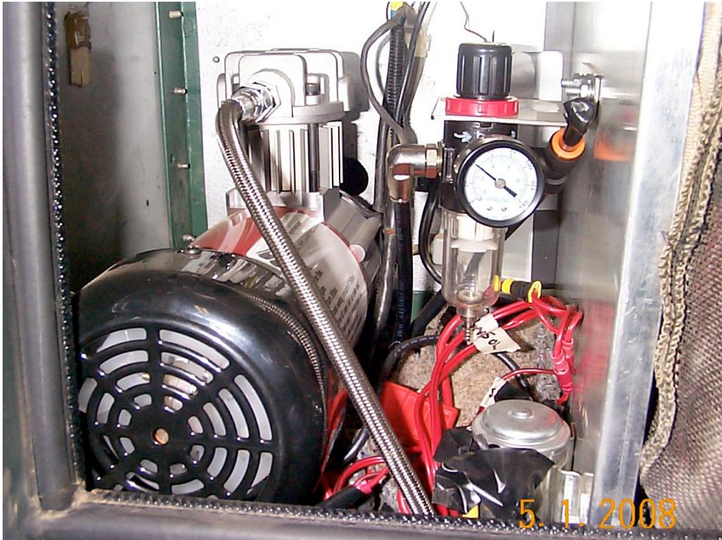
CTIS valve, Hummer tire pressure gauge, toggle for inflate/deflate and red switch for compressor
