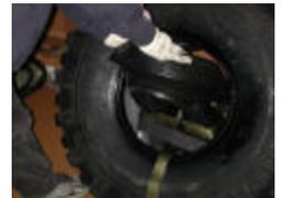
Using the brush provided swab the 'tire grease' (T) onto the VFI to ease the insertion and flip the tire over so that it rests and pushes on the runflat.
