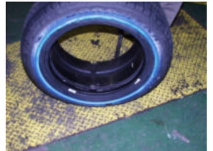
14. Examine the tire around the bead area to assure there are no cuts or gouges. After proper insertion is assured, carefully move the tire onto the next operation (Wheel Assembly)
