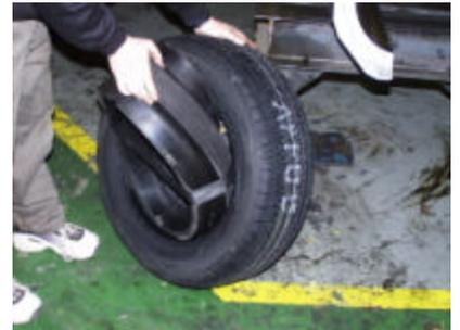
8. Turn the tire around and push the runflat into the tire as far as possible. Tire spoons can be used to expand the width of the tire to allow for the edges of the runflat to slide in past the beads.
