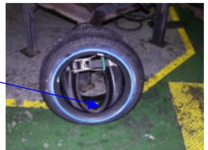
9. After the runflat has been carefully inserted as far as possible into the tire cavity, (as shown in the adjacent picture), go to step 10.
