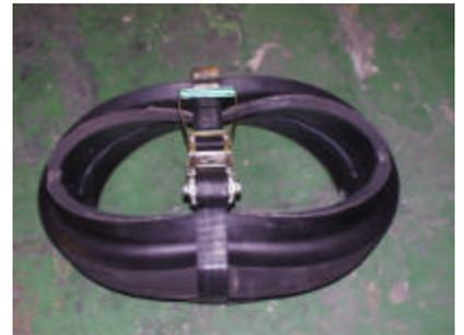
7. Position tire against a solid object such as a wall or rail. Insert the runflat device into the tire cavity as shown with the ratchet handle facing in towards the opening.
