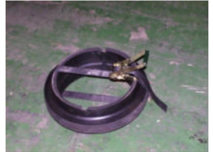
6. Utilize the ratchet to compress the runflat to less than half of the original inside diameter as shown, taking care not to pinch your fingers on the ratchet mechanism.
