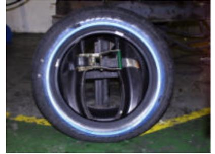
10. Lay the tire and runflat onto the floor with the ratchet handle facing up as shown. Press down on the tire to allow for the runflat edges to enter into the tire cavity as far as possible.
