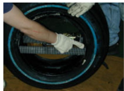
9. From the back side of the tire, insert the tire iron with the curved end up and over the runflat taking care not to damage the tire. The end of the tire iron should protrude past the other tire bead and rest in the runflat air slot.
