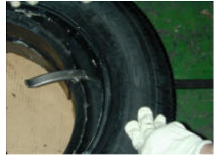
11. Place your foot on the tire iron and press down with steady pressure, while utilizing the ratchet (pulling towards you) to compress the runflat to less than half the original diameter. The tire will eventually begin to lift up and the runflat will begin to exit from the tire cavity.
