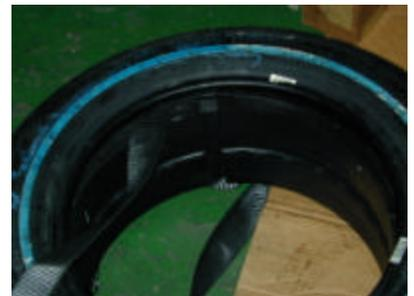
4. Roll the tire and runflat around so the portion of the strap you are feeding through can be pulled over top of the runflat.
