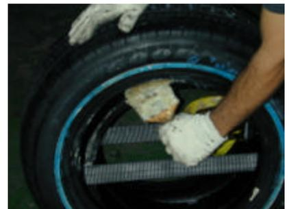
8. Center the runflat with the strap facing 3 & 9 O'clock as shown. Make sure the runflat is pressed as far to the bottom as possible.
