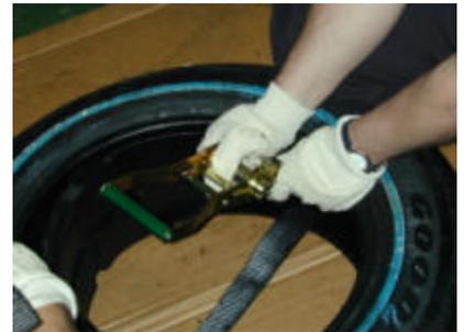
6. Feed the strap end through the ratchet hub barrel and pull tight. Ratchet the strap for about one turn.
