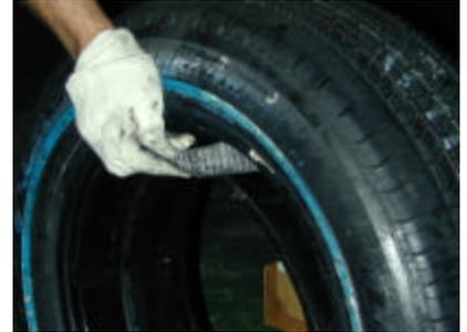
5. Align the strap opposite the two cross grooves in the bottom of the runflat. Grab the end of the strap and pull the lead end through the tire until the ratchet is pressed against the tire bead.
