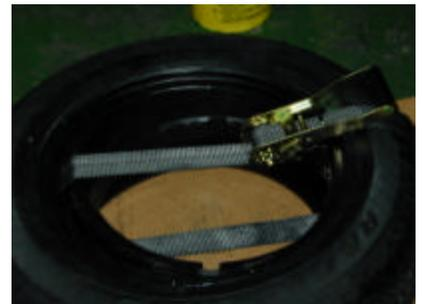
7. Liberally apply the tire lubricant to both beads at the top and bottom taking care not to put any on the strap itself.
