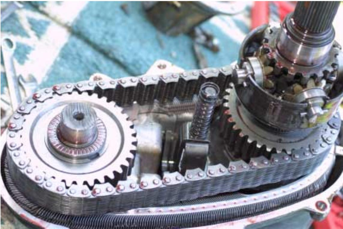
The above picture is of a military transfer case. Notice the cooling loop travels around the “drive gear and driven gear” location in the front case. The differential has large exposed gears (right upper).
