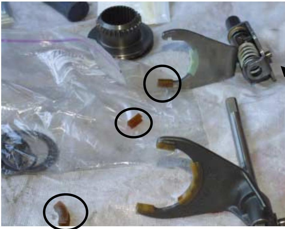
Each shifter fork has three plastic pads. The arrow identifies the pin
