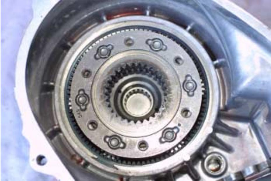
The outer annulus and inner assembly with the planet gears are now exposed, once the shifter mechanism is removed.
