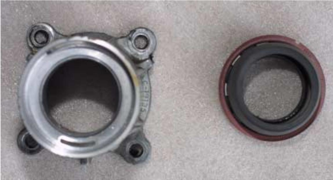
Next, remove the snap ring on the mainshaft that follows the rear housing bearing. Remove the bolts that hold the rear housing to the main case. There is sealant holding the machined surfaces together so gentle prying is usually required.
