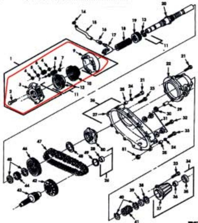
The differential assembly will allow for different wheel speeds when the transfer case is in the unlocked or high lock position.
