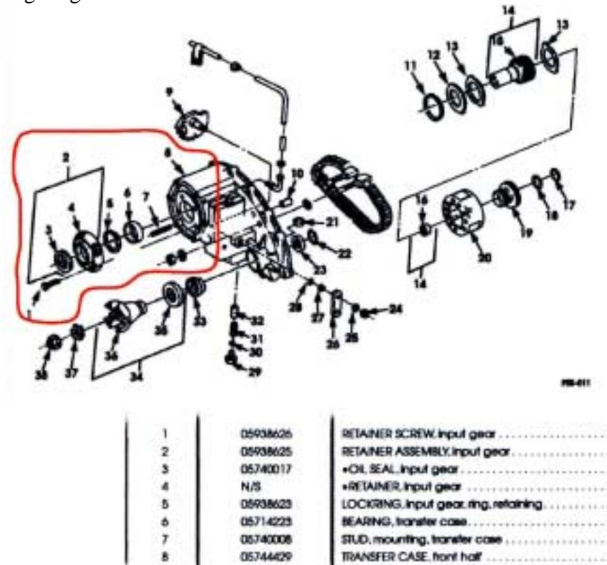
The Input Retainer assembly is where the transfer case physically connects to the transmission output shaft.
