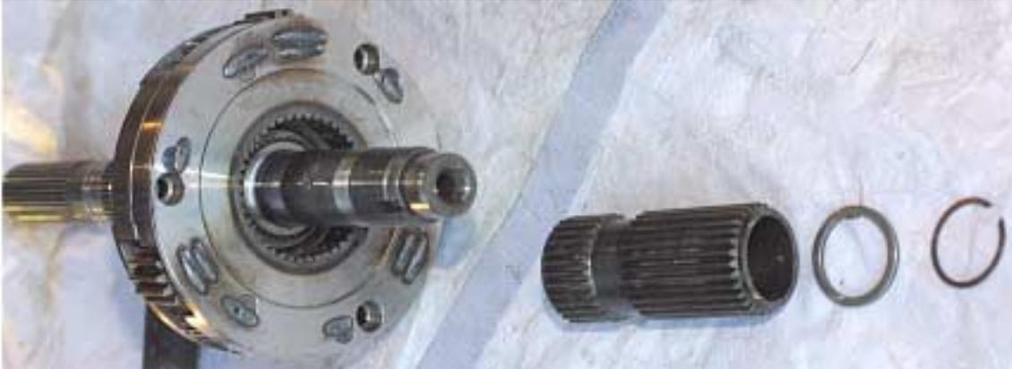
Remove the snap ring immediately prior to the differential assembly. The assembly can be removed from the mainshaft. Note: perform this in a clean flat work area for individual bearings will fall out upon separating the two components.
