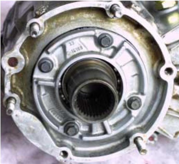
With the planetary assembly in the back portion of the front transfer case halve, the input gear retainer is attached to the forward portion of this case.
