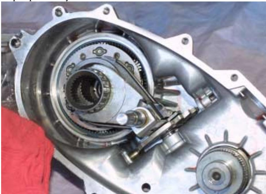
On the left is the input assembly with mode sleeve in place. To its immediate right is the shifter assembly. To the far right is the front output shaft assembly. The cooling loop has been removed. The slot at the 2:00 to 3:00 position holds a magnet. Immediately below, is the oil pump intake filter. (Removed)
