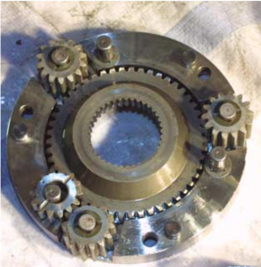
Thruster washers are placed on the bottom and the top of each long and short pinion gear. The short gears (7:00 position) have 16 individual bearings between the gear and the post of the differential case.
