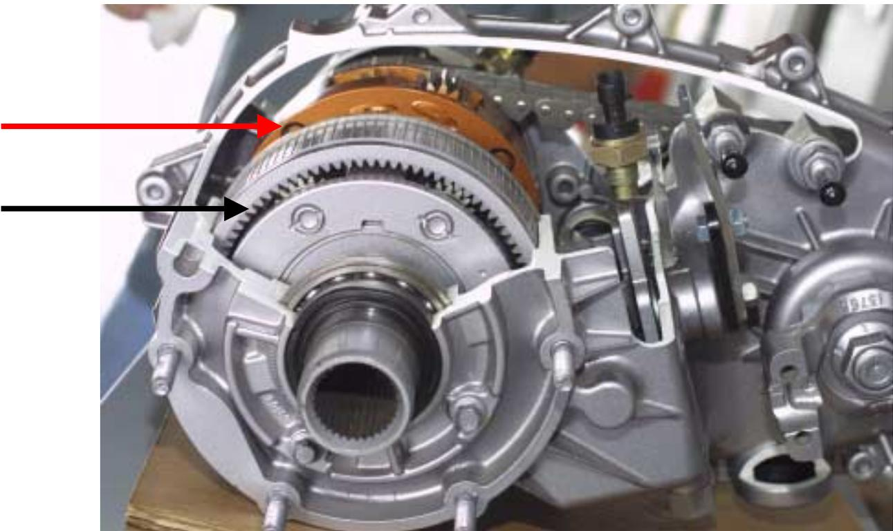
This is the civilian transfer case where the differential has a totally enclosed housing without gears visible. (red arrow). The black arrow identifies the planet assembly. The
