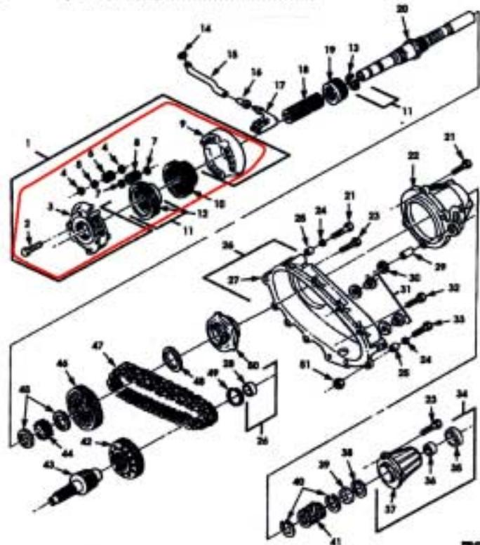
The differential assembly will allow for different wheel speeds when the transfer case is in the unlocked or high lock position.
