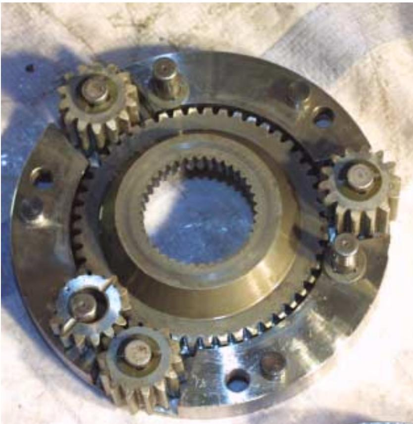
Thruster washers are placed on the bottom and the top of each long and short pinion gear. The short gears (7:00 position) have 16 individual bearings between the gear and the post of the differential case.
