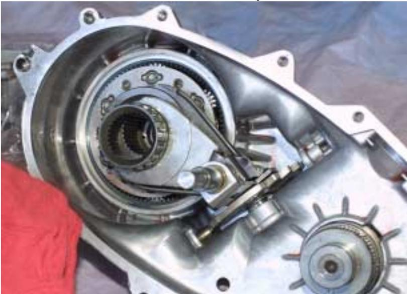
This shows both shifter arms (mode and range) with the corresponding sleeves in place on the shifter rail. The shifter arms slide down onto the rail and have a pin that inserts into slots on the sector plate.
