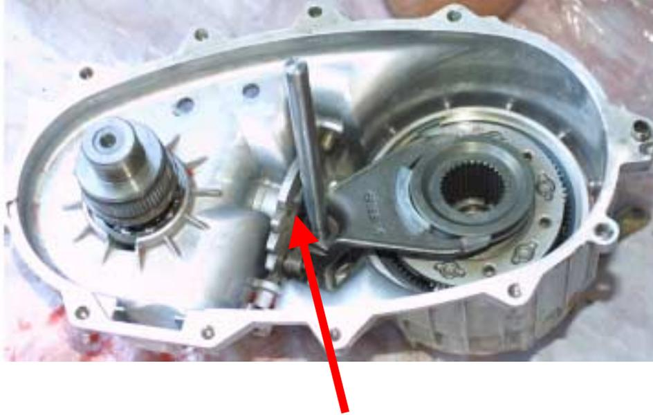
The upper slot in the sector plate for the mode arm pin is just visible. To remove the arms, you must manipulate the operating lever while twisting the arm to dislodge the pin. Once unengaged, the arm can slide away from the rail.
