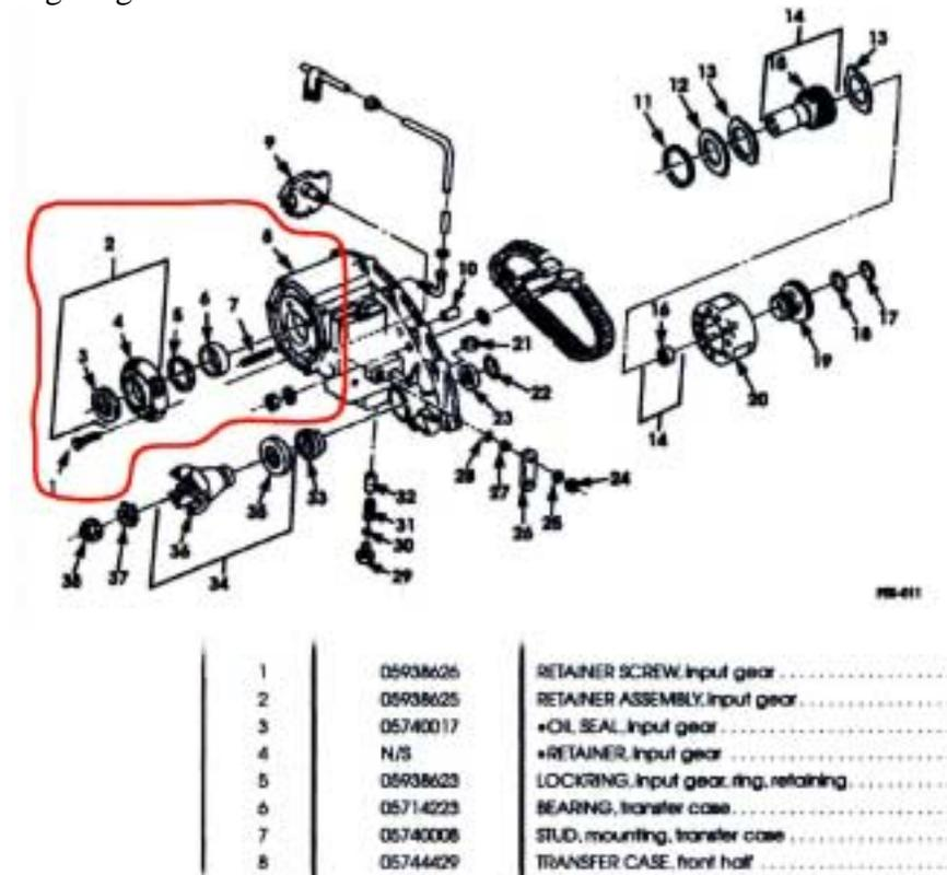
The Input Retainer assembly is where the transfer case physically connects to the transmission output shaft.
