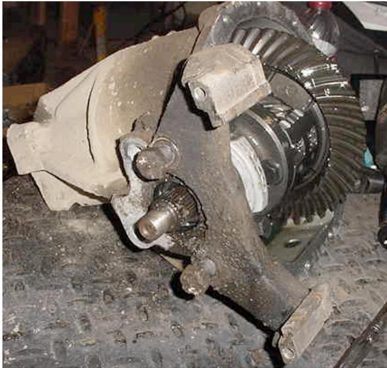
Caliper mounting brackets with the ring cover off
