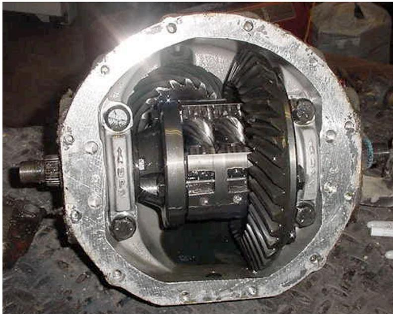
Torsen Differential with Ring Cover removed
