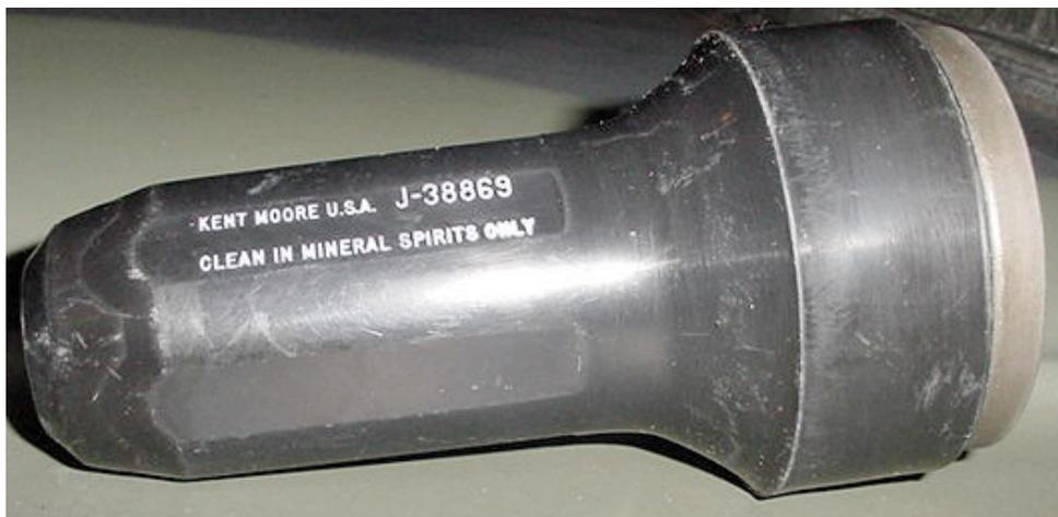
AMG Seal Installation tool with seal installed on it (PN J-38869)
