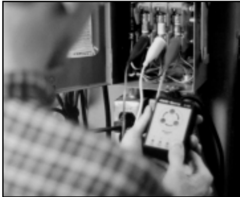
The Three-Phase Rotation Tester ensures properly wired motors, eliminating possible damage.
