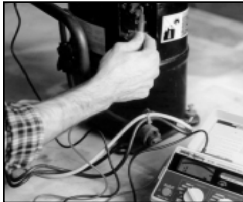
The Insulation Tester pressurizes electric wire to indicate whether or not insulation is good.
