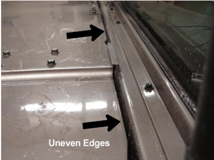
In Figure #4, the gap between the hood and the firewall is uneven.
