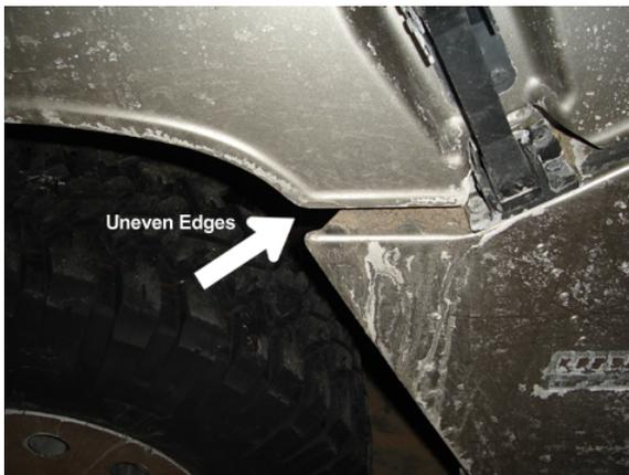
Figure #3 is a side view of the truck that reveals that the imaginary line arc from body to hood wheel well is out of alignment. The gap may also not be uniform along these surfaces.
