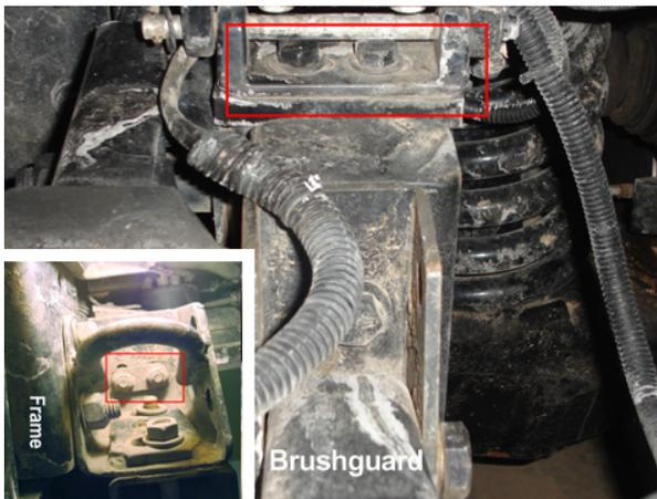
Figure #7 Illustrates the forward view of the alignment bolts and the insert on the lower left shows the corresponding nuts that are located under the truck in the center of the front hold down brackets.
