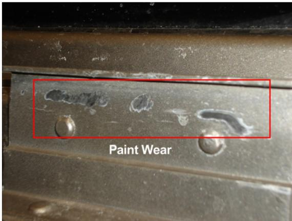
Figure #2 shows abnormal paint wear on the firewall from the hood impacting it while moving rearward during hard off-roading.
