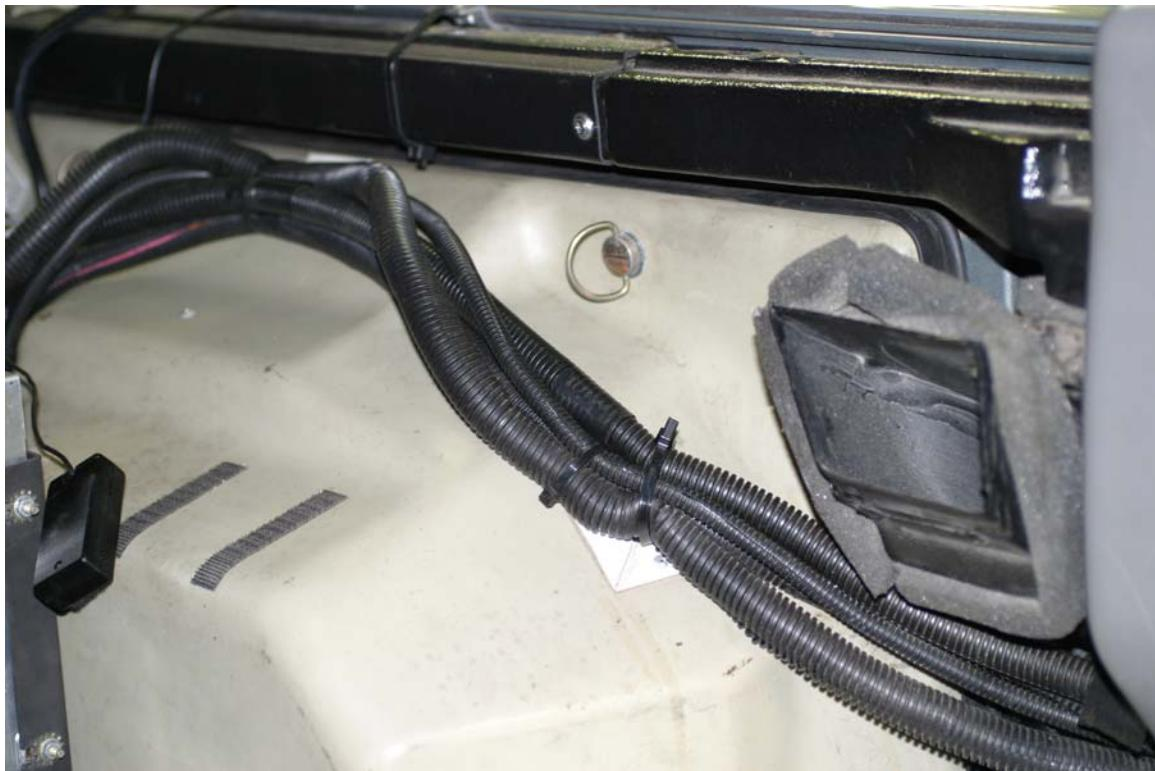
You can either disconnect the right side of the cable from the left by disconnecting the plugs or try to remove the doghouse with the cables intact.
