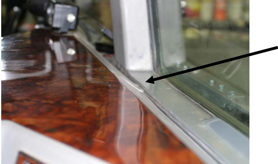
Remove the two 10mm bolts on either side of the console.
