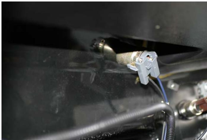
Detach the cables to the radio (1 – power, 1- antenna, and 4 speaker cables (2 – white, 2 – red)
