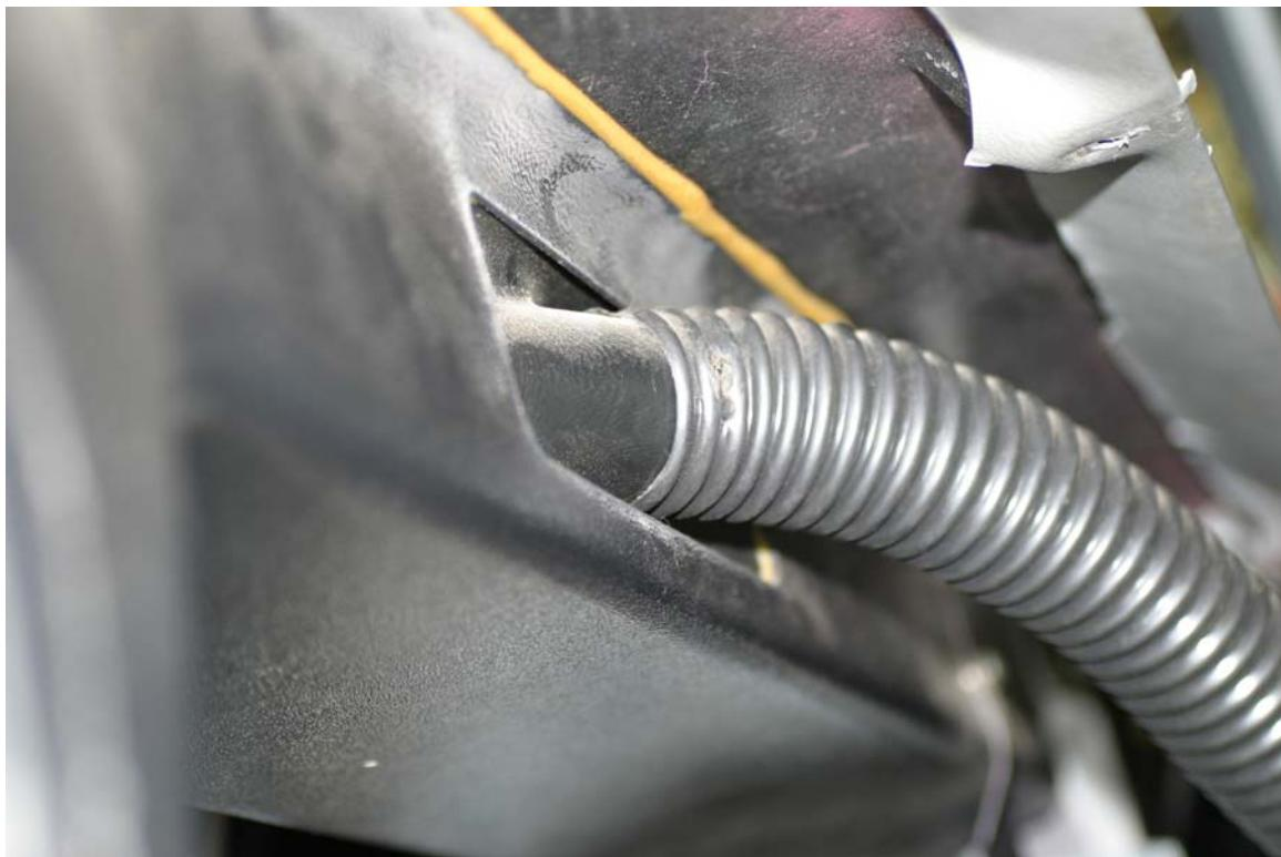
Remove the sheet metal screw to the vent hose and detach the hose from the console vent track.
