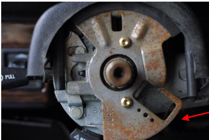
Lower column cover removed with the predrilled holes for the brush mechanism evident.
