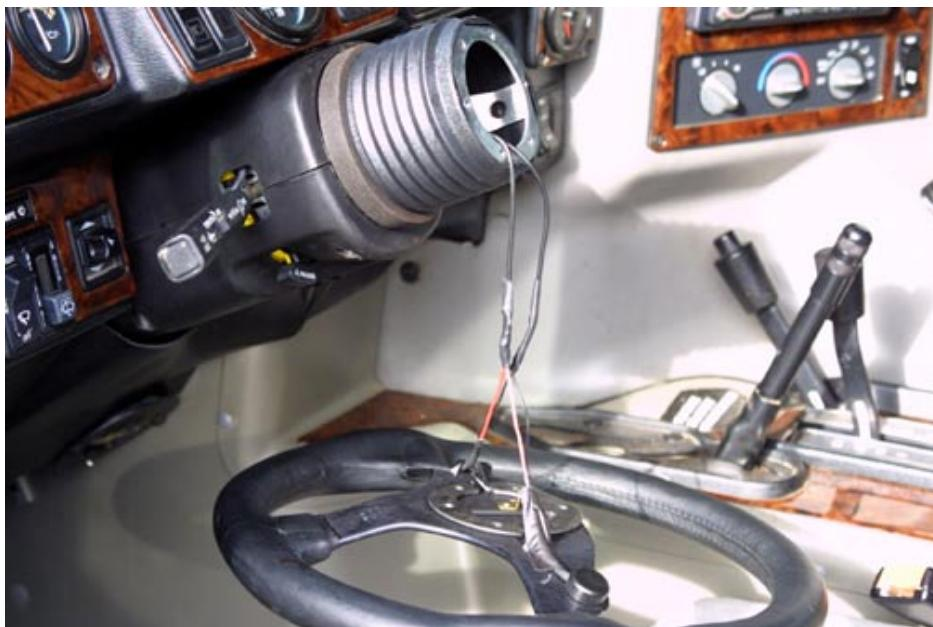
Finally, the steering wheel is attached to the adapter with the six Phillips recessed black screws.
